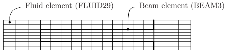
Figure 3.7: FEM mesh of part of the structure with the surrounding air.
